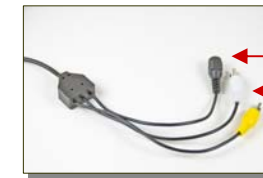
To AC adapter White Audio Out (to TV/VCR) Yellow Video Out (to TV/VCR)
